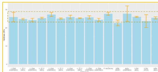
Also, in the scope of **finer characterization** resolution, dependable reduced elastic modulus and hardness were obtained in Continuous Stiffness Measurement (**CSM**) mode with a high sensitivity protocol. The result was achieved in **very low depth**, with the properties values being constant from a contact depth of about 10 nm in the fused silica reference sample.
